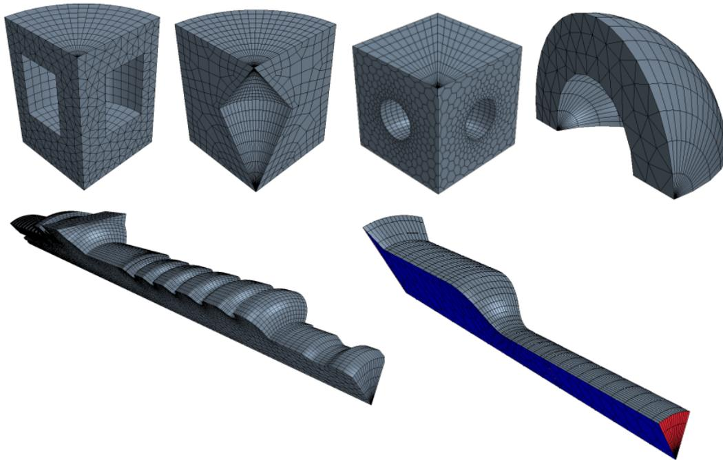
Fig. 4. Examples of volume meshes
