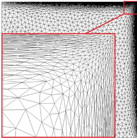
(a) Example of one anisotropic adapted mesh (5000 elements)
