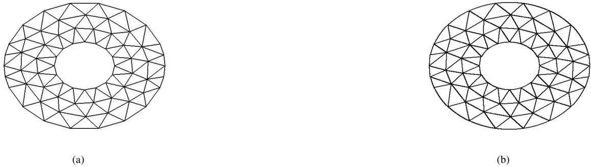
Fig. 1. An example showing (a) an initial linear mesh of the annulus; (b) a curved second-order mesh
