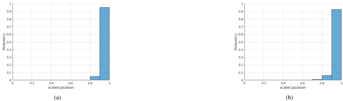
Fig. 3. Histograms of (a) the scaled Jacobian of the annulus example and (b) the scaled Jacobian of the airfoil exterior.
