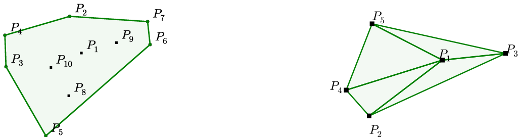
(a) Input sequence \mathcal{P} = \{P_1, \dots, P_{10}\} , and the output sequence \mathcal{C}^{\mathcal{P}} = \{=>, 2, 4, 3, 5, 6, 7, 2, <= \} representing its convex hull.
