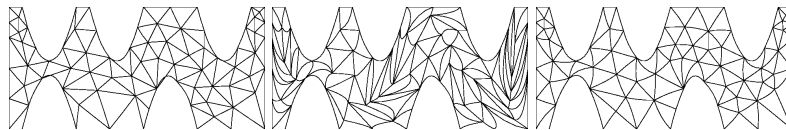
Fig. 4. Optimization of Triangle Meshes with Quadratic Finite Elements: Left: Initial 'Inverted'; Center: 'Non-inverted'; Right: Well-shaped
