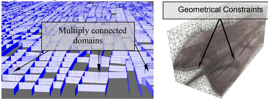
**Fig. 1.** Typical geological BREP geometry with multiple ( $N > 100$ ) domains: the CAD model (fractured stone) and hex-dominant mesh of the fault. Numerous CAD constraints make the boundary recovery difficult and induce large number of nodes and elements.
