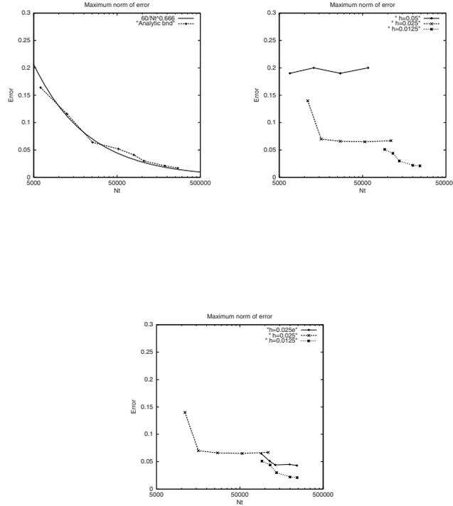
**Fig. 3.** Convergence analysis: using analytic representation of the obstacle boundary (top-left picture), using three discrete models  $\Gamma_{0.05}$ ,  $\Gamma_{0.025}$ , and  $\Gamma_{0.0125}$  for  $\partial B_{0.5}(0.18)$  (top-right picture), using the piecewise quadratic extrapolation  $\tilde{\Gamma}_{0.025}$  (bottom picture)
