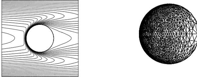
**Fig. 2.** Isolines of solution  $u_*$  in the plane passing through the center of the obstacle and parallel to the  $x_1x_2$ -plane (left picture) and the trace of a typical quasi-optimal mesh at the obstacle with analytic boundary (right picture)
