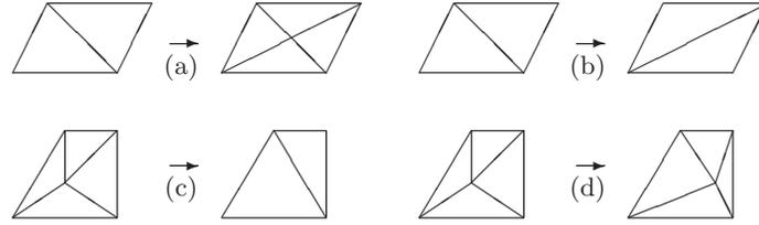
**Fig. 1.** Local topological operations for 2D triangular meshes: (a) node insertion, (b) edge swapping, (c) node deletion, and (d) node movement
