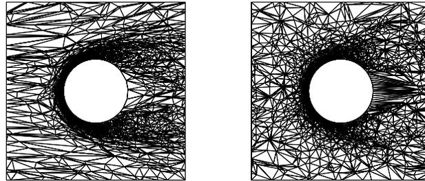
**Fig. 4.** The mesh cuts in the plane passing through the center of the obstacle and parallel to the  $x_1x_2$ -plane: The left picture corresponds to the case of analytic boundary representation. The right picture corresponds to the case of fixed-node constraints. The meshes have approximately the same number of elements ( $\sim 200k$ )
