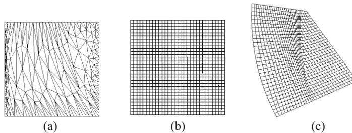
**Fig. 5.** (a) Triangulation of the new parametric domain obtained by parametrization of the surface triangulation shown in Fig 4 (b); (b) Structured grid on the new parametric domain; (c) Corresponding structured grid on the surface obtained using the new parametrization mapping.
