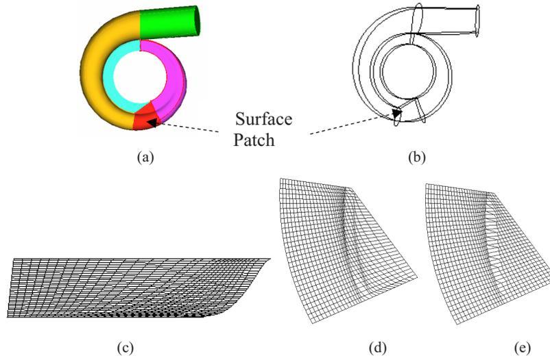
**Fig. 3.** Singular surface patch of a volute. (a), (b) The patch shown as part of the volute; (c) TFI grid over the trimmed parametric domain of the patch; (d) Corresponding structured grid over the face; (e) Grid obtained by TFI in 3D and projection.
