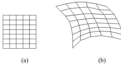
**Fig. 2.** (a) Structured grid over the parametric domain  $D$ ; (b) Corresponding structured grid over the surface  $S$ .
