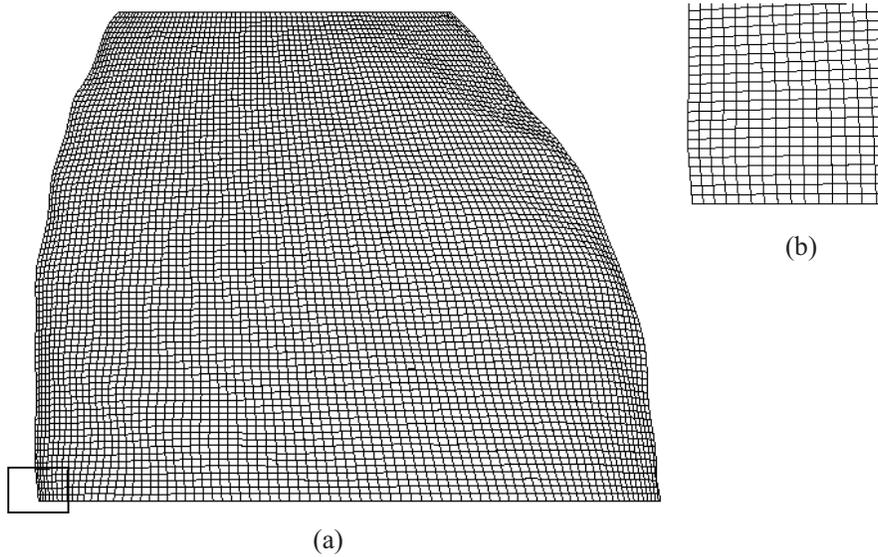
**Fig. 8.** (a) Structured grid over the four-sided patch of the human lung model obtained using the parametrization; (b) zoomed-in view of the lower left corner.
