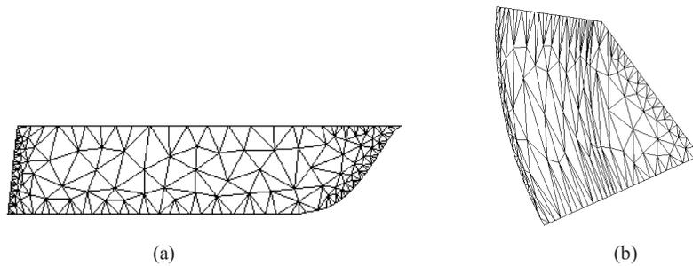
**Fig. 4.** (a) Triangulation of the original parametric domain; (b) Corresponding triangulation of the surface patch.
