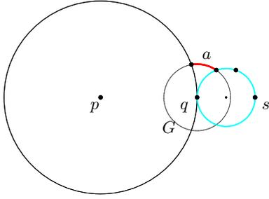
**Figure 2:** The gate sphere of  $q$  for the given segment  $(q, s)$  is shown as  $G$ . The gate arc of  $q$  is shown in bold as  $a$ .
