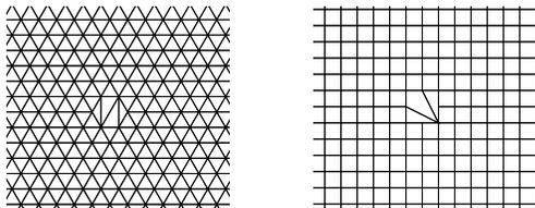
**Figure 7:** Zoom on the initial regular grids with one node removed.
