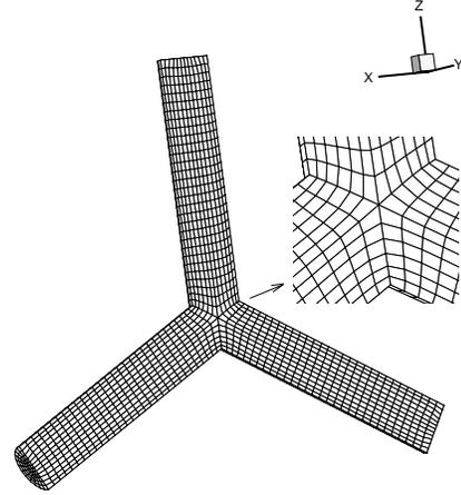
**Figure 11:** Grid slice after smoothing with  $\theta = 0.8$ .
