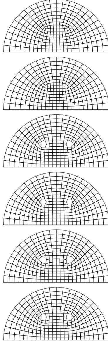
**Figure 6:** From top to bottom: whole smoothed grid, smoothed grid with free nodes on the boundaries of deleted patches, smoothed grid with patch boundaries fixed from initial grid, smoothed grids with vertex angle  $\chi$  equal to 120, 80 and 90 degrees.
