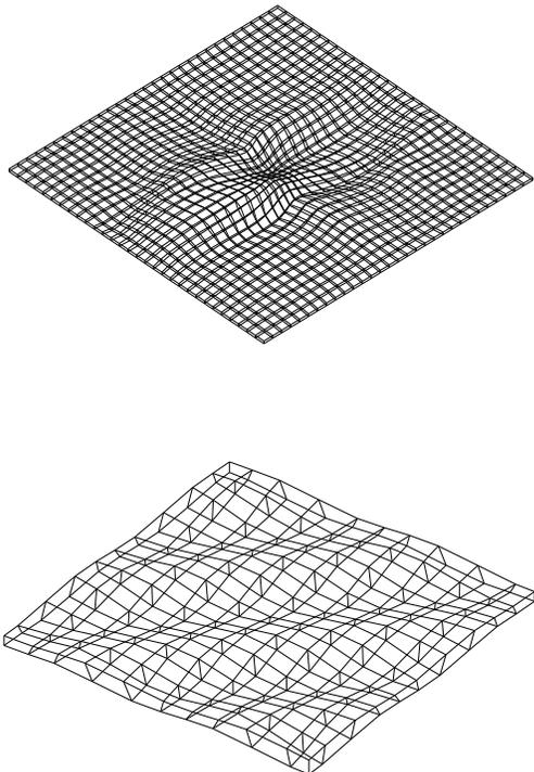
**Figure 13:** On top: adaptation to  $u = \exp\left(-\frac{|x-0.5|+|y-0.5|+|z-0.5|}{\epsilon}\right)$ , on bottom: adaptation to  $u = \sin(2\pi(x + y + z))$ .
