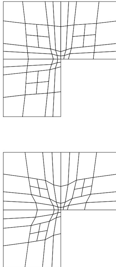
**Figure 14:** Adaptive smoothing step, on top: grid before smoothing, on bottom: smoothed grid.
