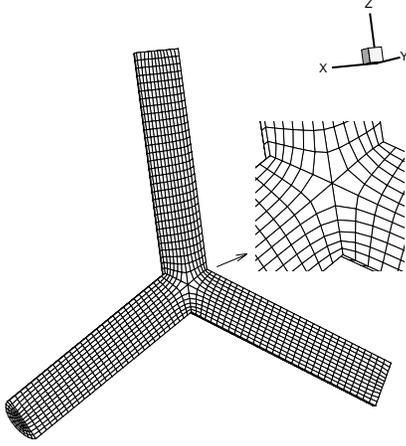
**Figure 12:** Grid slice after smoothing with  $\theta = 0.2$ .
