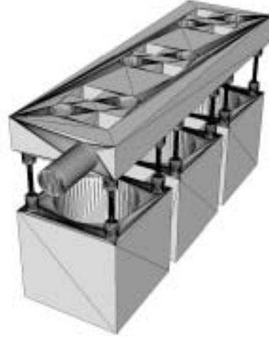
Figure 7: Water jacket — Triangulated geometry [25].
