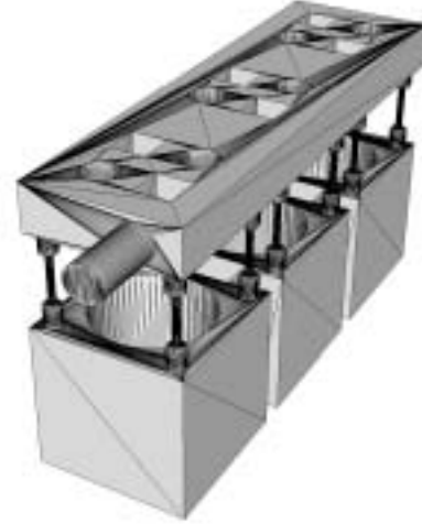
Figure 7: Water jacket — Triangulated geometry [25].
