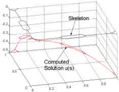
Figure 5-3: Computed solution on the skeleton of a modified L-bracket.
