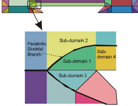
**Figure 3-5: S-Voronoi decomposition of dovetail.**
