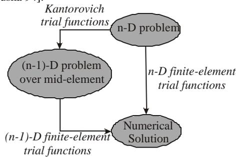
**Figure 1-2: Mid-element dimensional reduction.**
