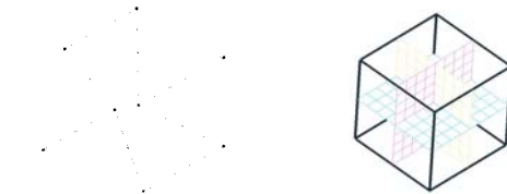
Figure 3. Topology corners displaced, but it produces the same grid
