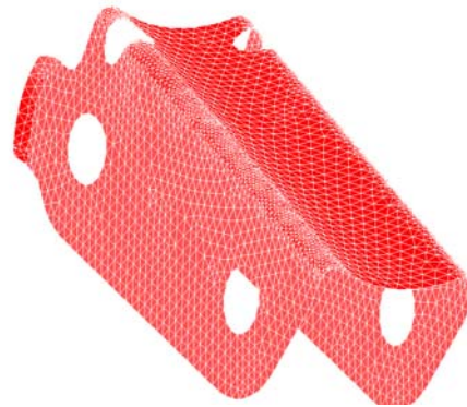
Figure 10c – 3D final mesh
