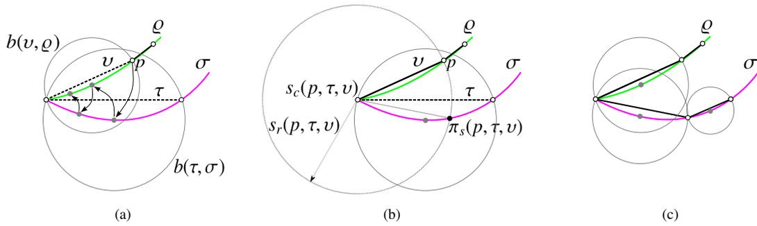
Fig. 2: (a) Mutual encroachment of 1-simplices  $\tau$  and  $\nu$  caused by a sharp feature of 1-cells  $\sigma$  and  $\rho$ . (b) Encroached restricted 1-simplex  $\tau$  and sphere of projection  $s(p, \tau, \nu)$ . (c) Result of refinement by circular projection  $\pi_s(p, \tau, \nu)$ .
