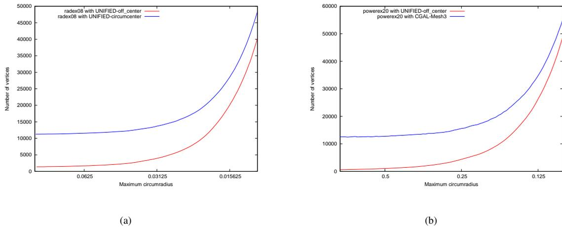
Fig. 4: Comparison of number of vertices as a function of maximum circumradius. (a) PLC device radex08. (b) PSC device powerex20.
