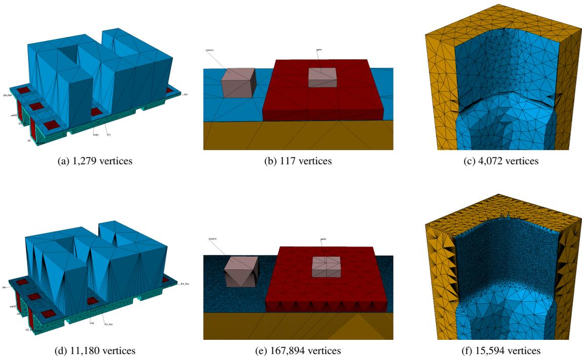
Fig. 3: Comparison of number of vertices for radex08, powerex18 and powerex20 devices. (a), (b), (c) UNIFIED-off\_center. (d), (e) UNIFIED-circumcenter. (f) CGAL-Mesh3.
