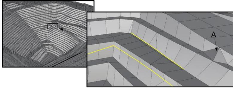
Fig. 4. Open pit mine meshed with Griddle. Edge A required manual swapping to correct ramp geometry. Yellow lines indicate trace of a fault that intersects the geometry. Upper yellow edges were manually collapsed onto adjacent ramp edges to eliminate sliver elements in the volume mesh.
