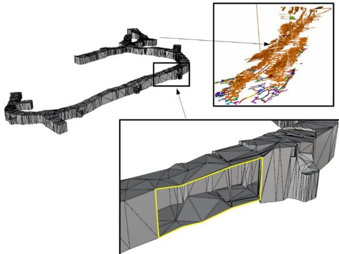
Fig 2. As-built tunnel geometry provided by a mine. Detailed view (lower right) showing portion of a tunnel surface mesh. Yellow boundary outlines area that has been opened intentionally to allow viewing of the interior of the tunnel mesh. Note the extraneous facets on the inside.
