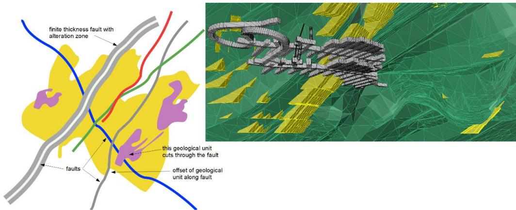
Fig. 1. Hypothetical cross-section of geology and structures (left) and actual mine and geological structure geometry (right). In the left view, the yellow and purple areas represent areas of different ore that are cross cut by faults, some with finite thickness. Faults are not always continuous, as shown by the red fault that terminates in the yellow ore body.
