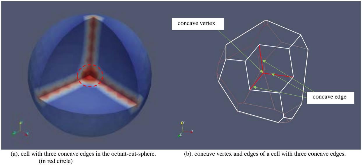
Fig. 4. The octant-cut-sphere model and the cell with three concave edge.
