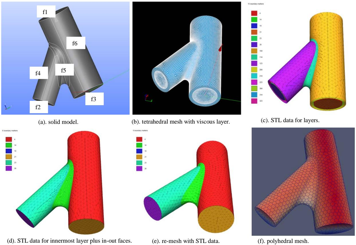
Fig. 12. mergedPipes model and tetrahedral mesh generation.
