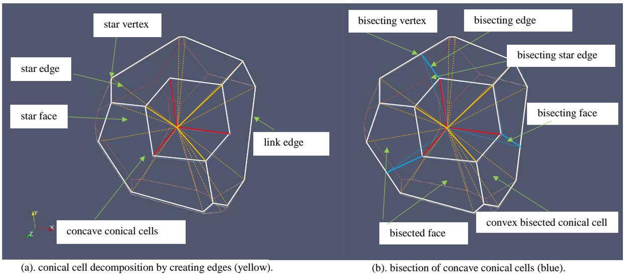
Fig. 5. Conical cell decomposition and bisection process.
