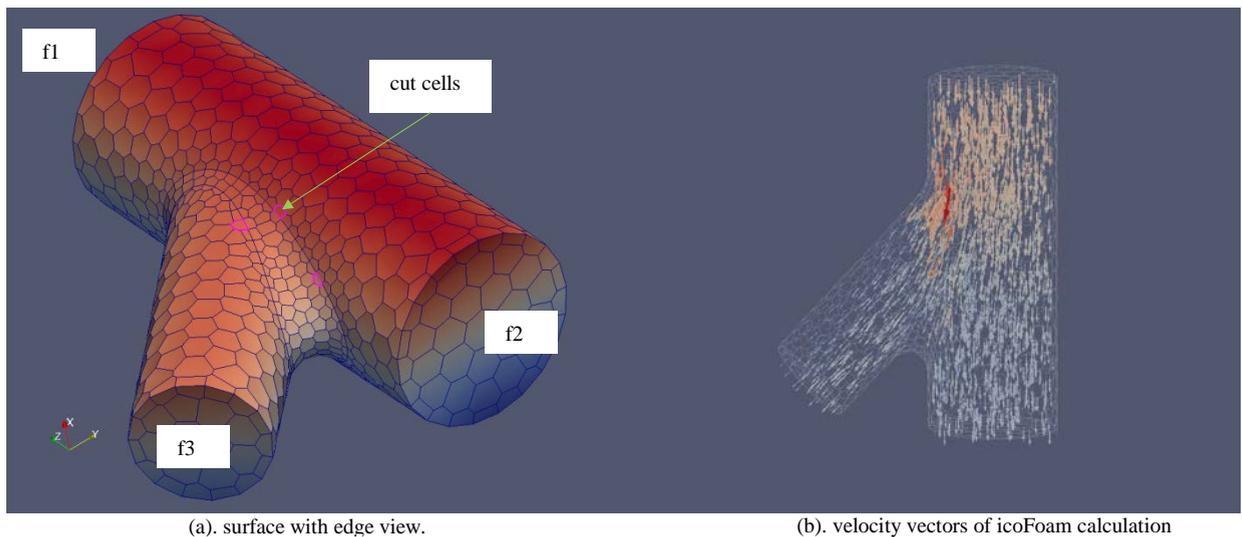
Fig. 9. Polyhedral mesh of mergedPipes model with fillet.
