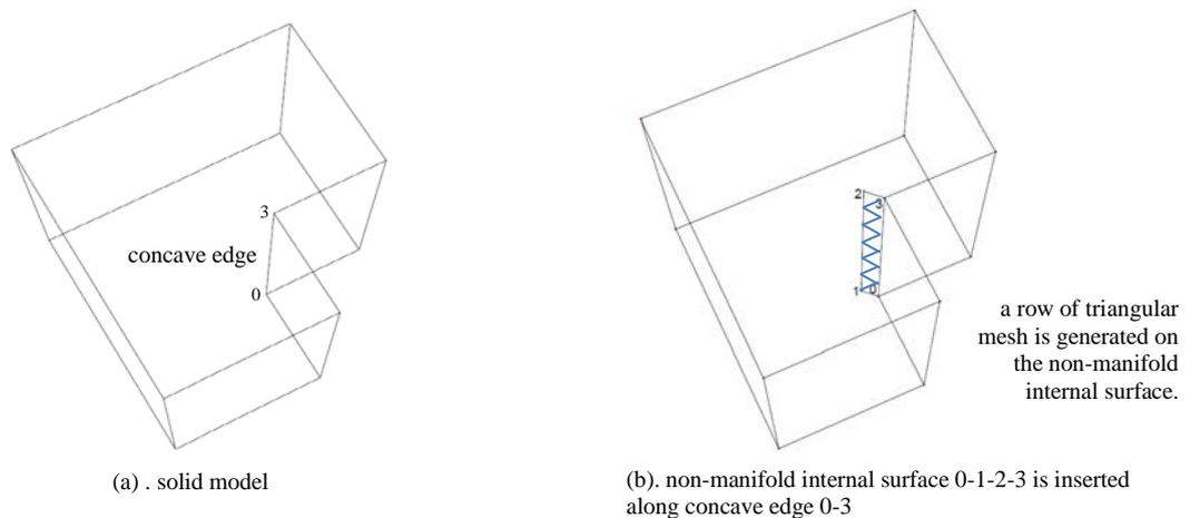
Fig. 1. cavityClipped model with a non-manifold surface.
