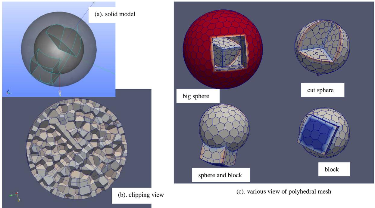
Fig. 11. Polyhedral mesh of the model A-Shape.
