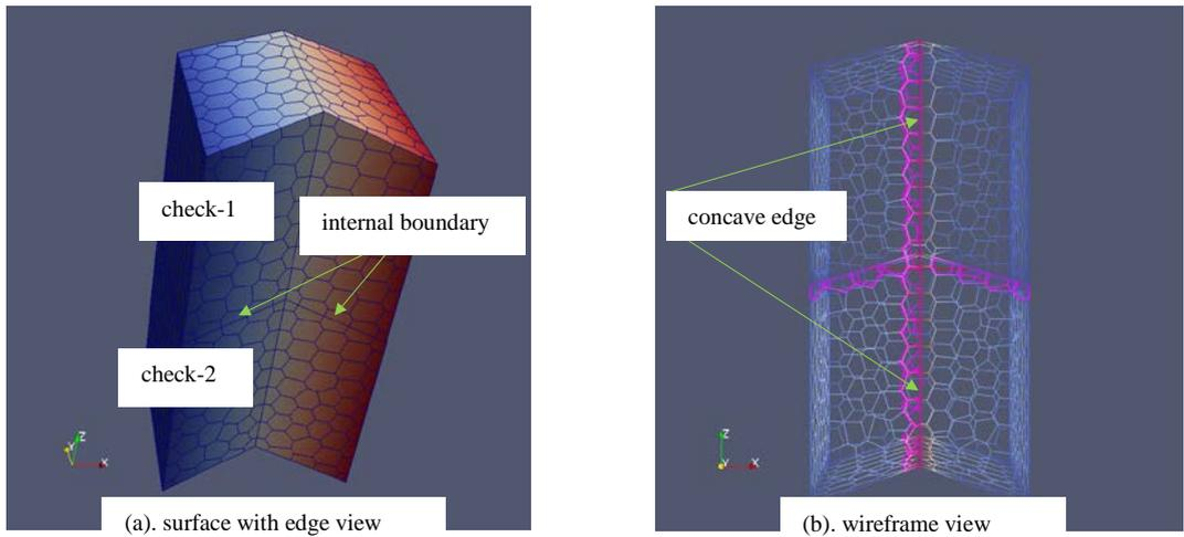
Fig. 10. Polyhedral mesh of the mergedChecks – internal boundary test.
