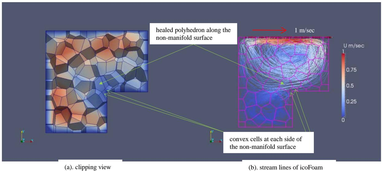
Fig. 3. Polyhedral mesh of cavityClipped model.
