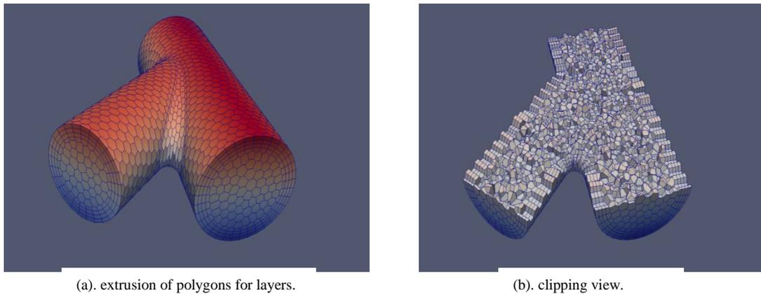
Fig. 13. Polyhedral mesh of the mergedPipes with polygonal prism viscous layers.
