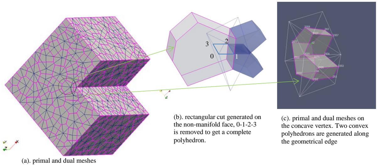
Fig. 2. Construction of convex cells on cavityClipped model.
