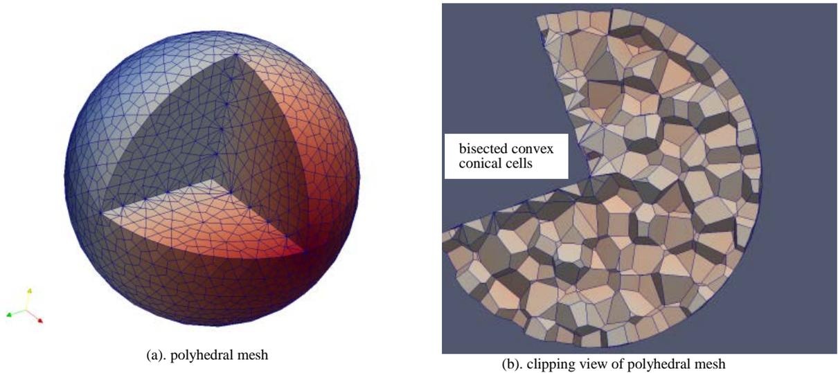
Fig. 6. Polyhedral mesh of the octant-cut-sphere.
