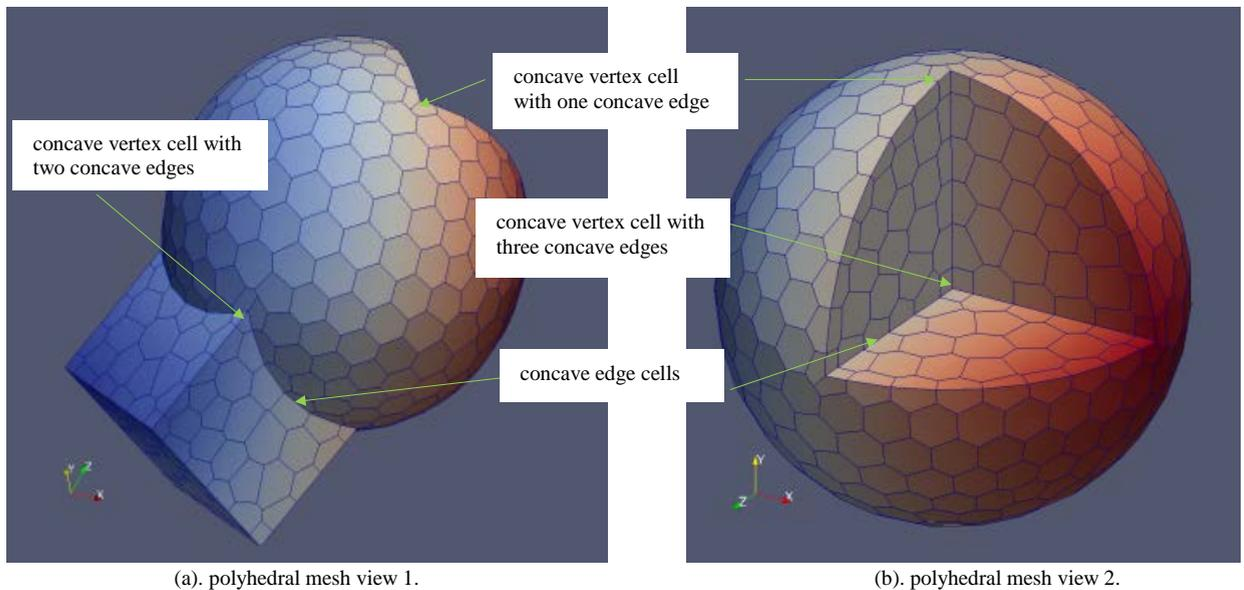
Fig. 7. Polyhedral mesh of the octant-cut-sphere-block-merge.
