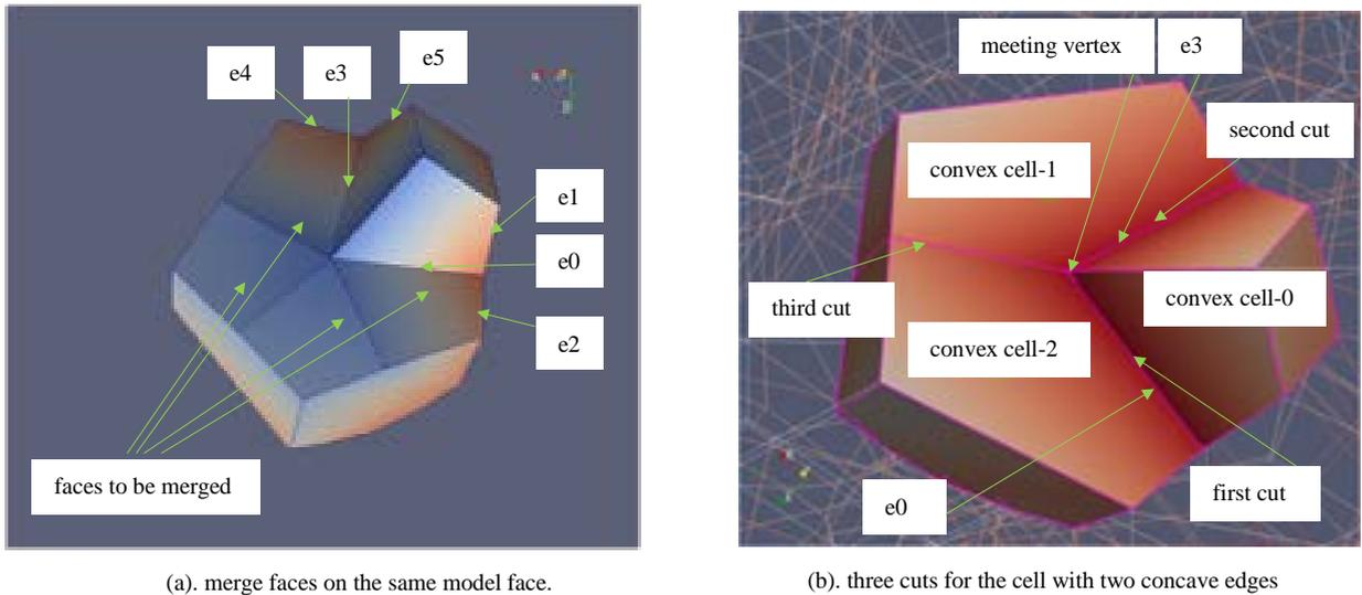
Fig. 8. Cutting process of the concave vertex cell with two concave edges.
