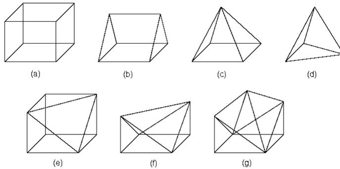
Fig. 2. The seven final elements of the  $\Omega$  Mesh Generator: (a) Cuboid, (b) Triangular Prism, (c) Quadrilateral Pyramid, (d) Tetrahedron, (e) Tetrahedron Complement, (f) Deformed Prism, and (g) Deformed Tetrahedron Complement.
