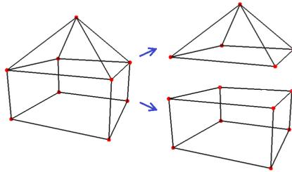
Fig. 5. Generic #9 element and its separation into two different elements.
