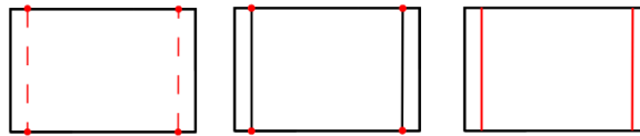
Fig. 7 Virtual Topology relationships: (a) Virtual model, (b) Ignored vertices in host model, (c) Ignored edges in host model
