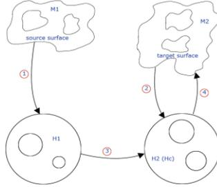
Fig. 1. Road map for mapping all-quad mesh from the *source* surface to the *target* surface.
