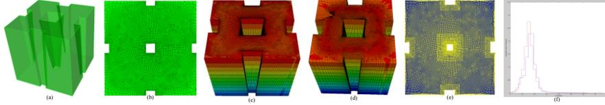
**Fig. 3.** Sweep volume with concavities and varying square holes: (a) the 3D model; (b) the *source* mesh (c) an all-hex mesh by our method; (d) an all-hex mesh from *Cubit* 12.2 which contains a lot of inverted elements; (e) an all-hex mesh from linear method which contains many inverted elements; (f) the mesh quality histogram for the result from our method(blue) and *Cubit* 12.2(red)
