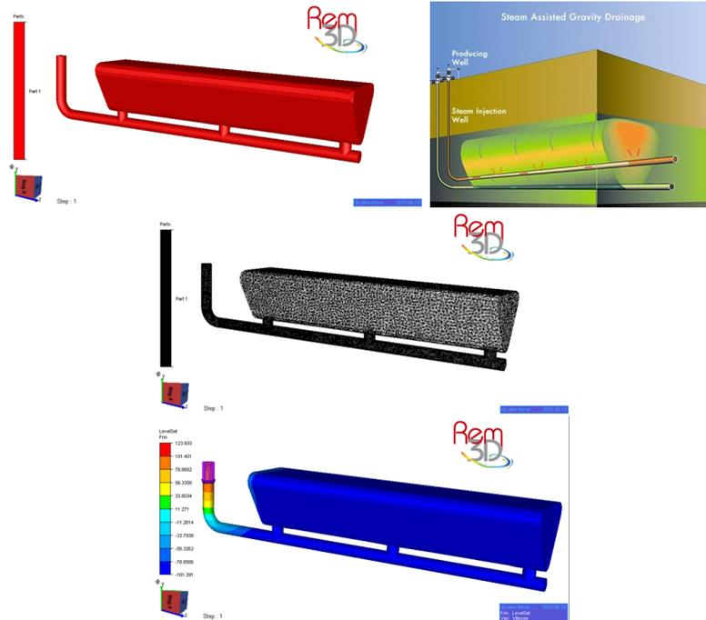
Fig. 1. SAGD CAD, configuration, mesh and point injection
