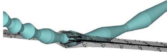
**Figure 11. Streamlines of the flow past the tube**
