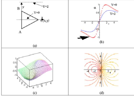
**Figure 2.  $\alpha$  for a triangle. (a) A triangle with point C perturbed over the x-y plane. (b) The change of  $\alpha$  on  $y=0$  and  $y=2$ . (c) The 3D plots of  $\alpha$ ; (d) the contour of  $\alpha$  on the x-y plane**
