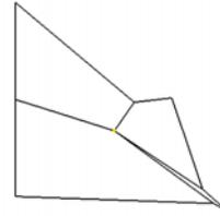
Figure 20 a Test quadrilateral configuration with the center node being smoothed
