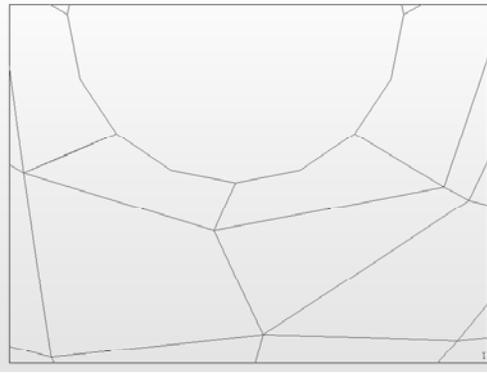
**Figure 1. A simple mesh with poor smoothing**
