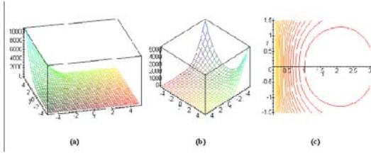
**Figure 7. the penalty term and the objective function (a) the penalty term when considering only one side of the triangle, (b) the final shape of the objective function, (c) the contours of the final objective function in the feasible region.**
