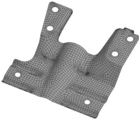
Figure 18. example surface mesh
