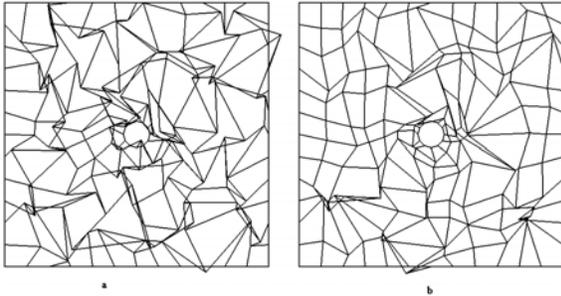
**Figure 14. untangling, initial mesh and first iteration mesh**
