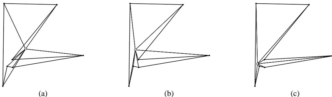
Figure 5: Comparison of smoothing methods. (a) Laplacian. (b) Angle-based [21]. (c) Weighted angle-based.
