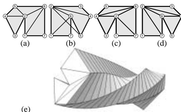
**Figure 1: The concept of compatible triangulations of corresponding polygons. Vertex correspondence is denoted by digits. (a),(b) Non-compatible triangulation. (c),(d) Compatible triangulation. (e) The sweep with bases (c) and (d).**
