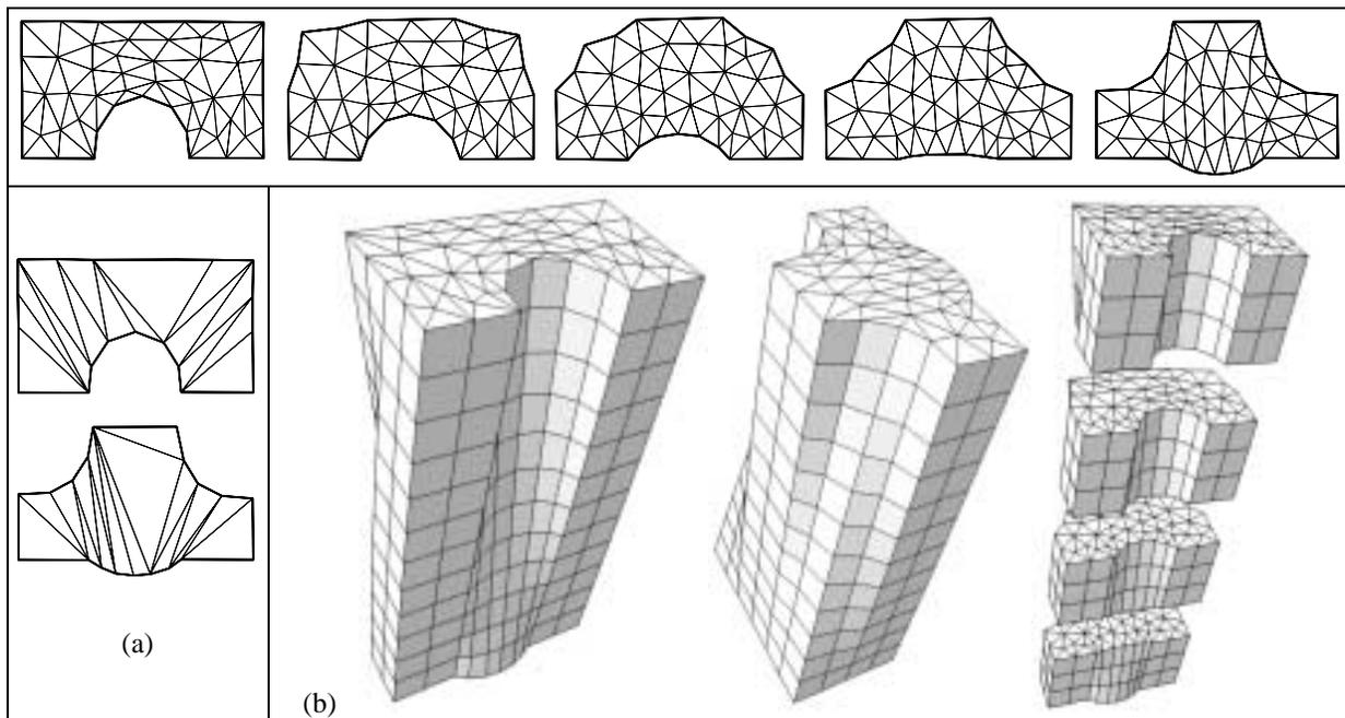
**Figure 9: 3D sweep generation. (a) Optimal (no Steiner vertices) compatible triangulation of source and target polygons. Top row: High-quality compatible triangulation and intermediates generated by morphing procedure. Minimum angles of the source and target triangulations are 27.2° and 25.9°, respectively. (b) 3D visualization of sweeps from a number of different angles.**
