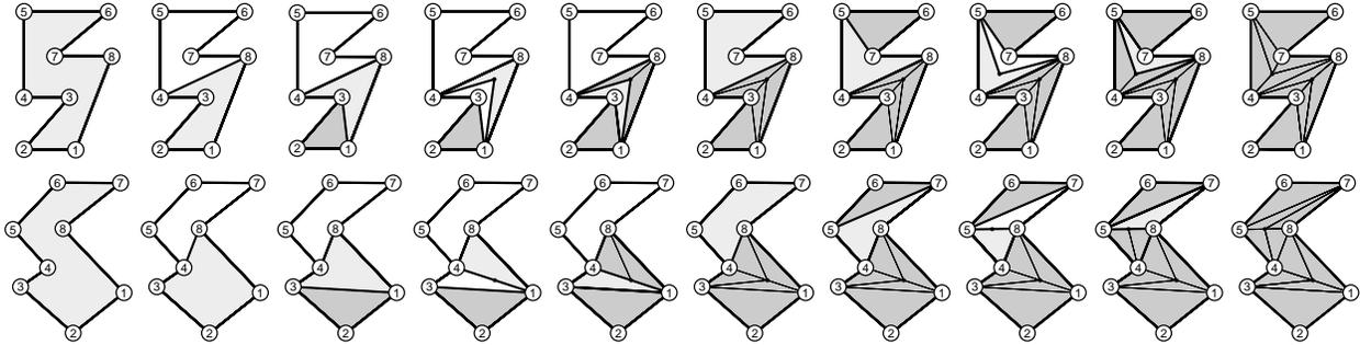
**Figure 3: Compatible triangulations of two polygons (one on each row), whose vertex correspondence is denoted by digits. The light grey region denotes the current polygon during the recursion. The grey regions are regions already triangulated. Thick segments are minimal-link polylines, which recursively partition the polygons.**
