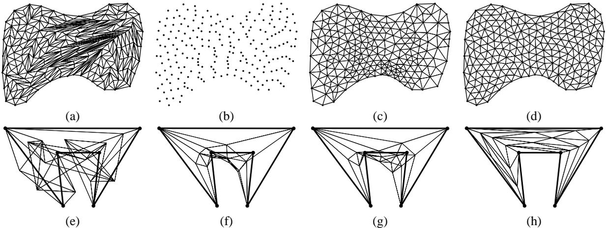
**Figure 7: Area-based remeshing. (a) Triangle areas of the mesh from Figure 6 are equalized. (b) Discarding the edges of (a) reveals a uniform vertex distribution. (c) Mesh obtained by alternation of angle-based smoothing and weighted angle-improving edge-flips. (d) Mesh obtained by alternation of area equalization and edge-flips. (e) A polygon with random distribution of interior vertices. (f) Laplacian smoothing of (e). (g) Angle-based smoothing of (e). (h) Area equalization of (e).**
