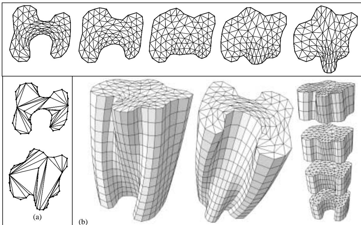
**Figure 10: 3D sweep generation. (a) Compatible triangulation of source and target polygons with three Steiner vertices. Top row: High-quality compatible triangulation and intermediates generated by morphing procedure. Minimum angles of the source and target triangulations are  $15.9^\circ$  and  $15.3^\circ$ , respectively. (b) 3D visualization of sweeps from a number of different angles.**
